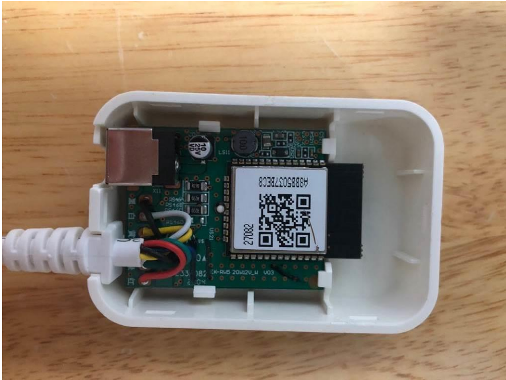
PCB of control box
